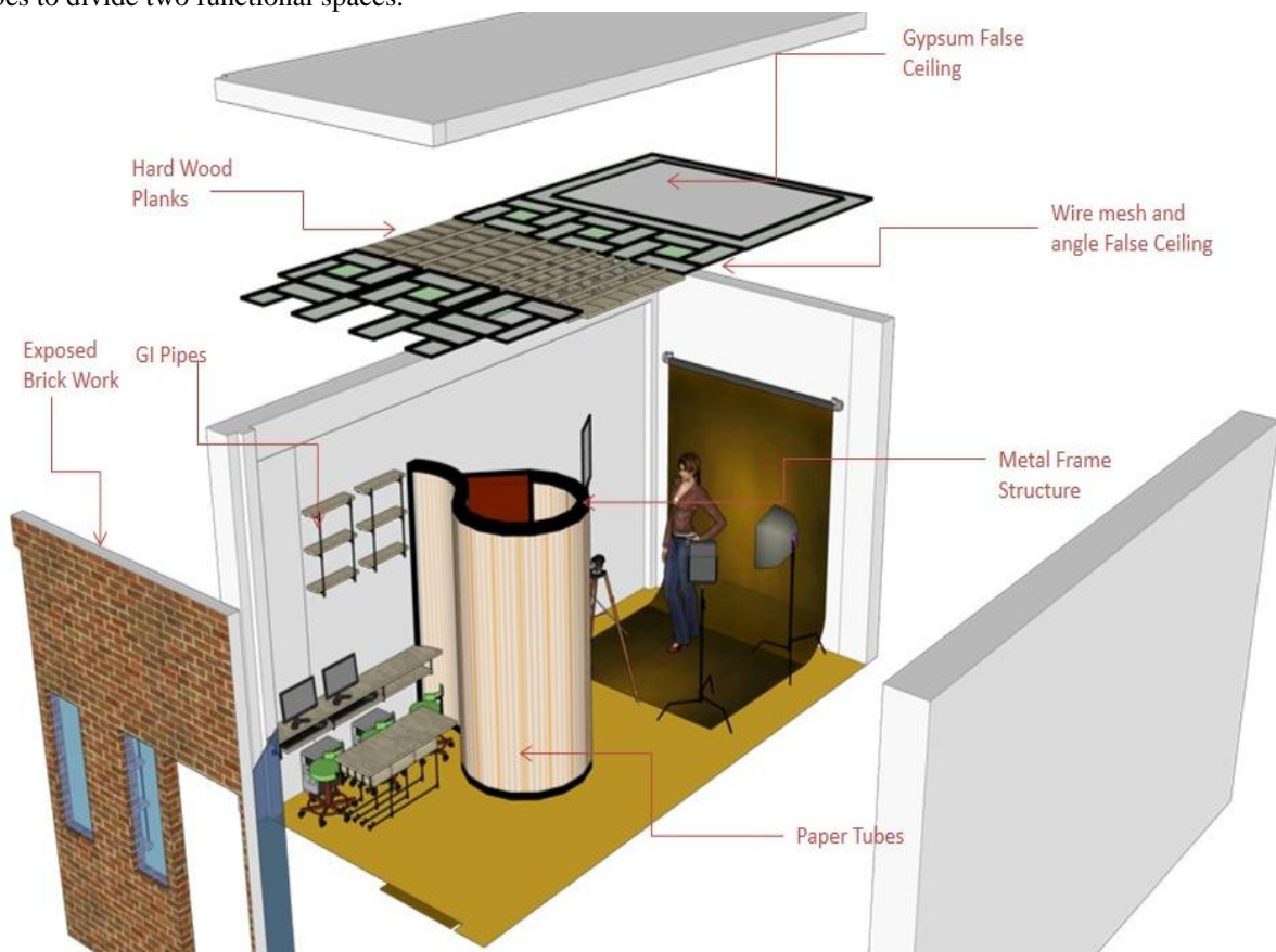
Figure 8: Conceptual view of photo studio showing S partition made in mild steel frame and paper tubes
