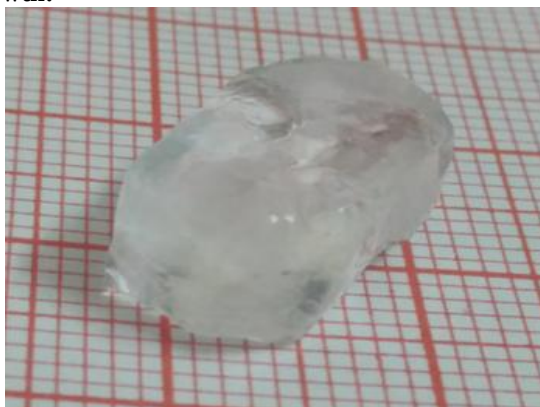
Figure 1: Photograph of the grown urea cadmium sulphate crystal
