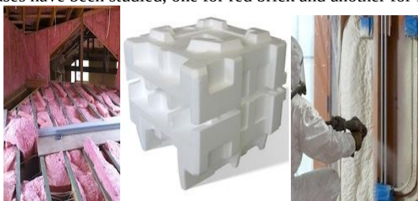
Figure 1: (i) fiber glass (ii) polystyrene (iii) polyurethane foam [21]
